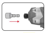
3. Release the drive bit chuck sleeve then pull on the bit to ensure it is firmly in place.
